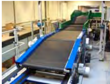
Figure 6. A toploader, where bags arrive on a traditional conveyor belt
